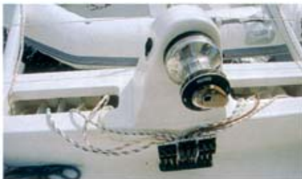
The main is hoisted from the cockpit thanks to the electric winch. The rope box and set of jammers are well thought out for peace of mind cruising.
