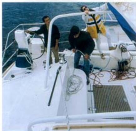
The main is hoisted from the cockpit thanks to the electric winch. The rope box and set of jammers are well thought out for peace of mind cruising.
